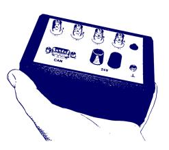
The **Mini**MessBOXes can be optionally equipped with measuring inputs for temperature sensors, for strain gauge sensors or for active sensors (0/4 ... 20 mA or ± 10 V). Each MiniMessBOX can be adapted variably according to customer requirements, whether 1, 2, 3 or 4 channels.
